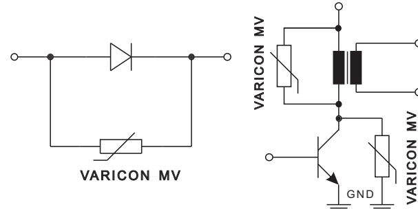
(c) Stabilizing voltages and absorbing line surges
