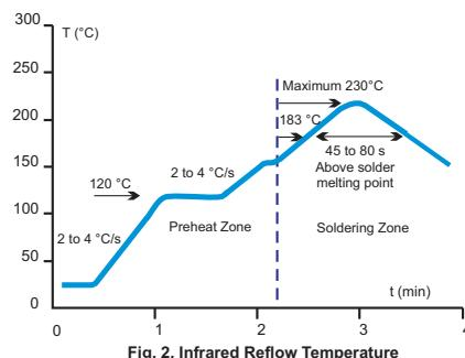
Fig. 2. Infrared Reflow Temperature Profile for Pb-containing Soldering
