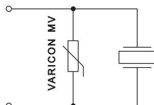
(h) Elimination of static electricity from circuits
