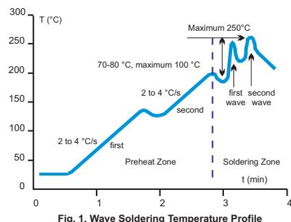
Fig. 1. Wave Soldering Temperature Profile for Pb-free and Pb-containing Soldering
