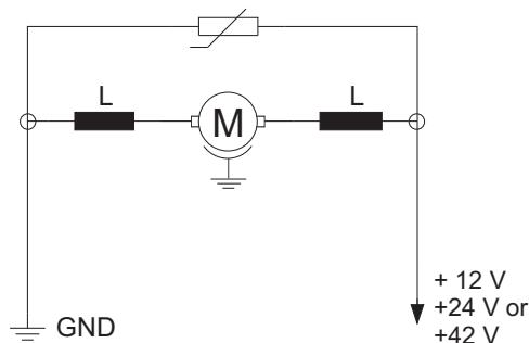
Provides for the elimination of transients and EMI noise in automotive electronics such as engine control, exhaust gas control, safety systems, etc. against disturbances caused by small motors used in automobiles. Most frequently, small motors in an automobile are those used for windscreen wipers, window mechanisms, seat adjustments and automatic door locking.
