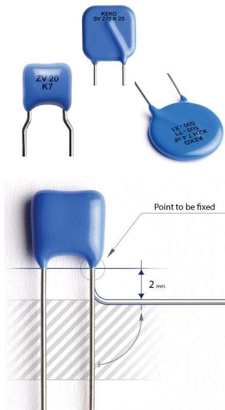
Very often before soldering through-hole components, their leads get bent. It is important not to damage the component during lead bending. Typical damage incurred during bending is cracks in epoxy parts, which can lead to increased humidity sensitivity of a component and consequently to a shorter life time.
