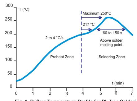
Fig. 3. Reflow Temperature Profile for Pb-free Soldering
